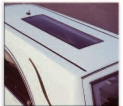
Standard skylight to illuminate casket area.
