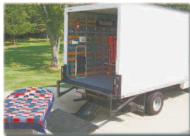
Professional Transport Service's bariatric removal vehicle, showing the oversize transport cart and lift.
