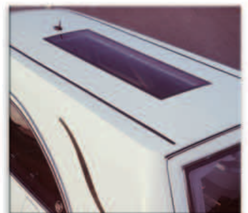
Standard skylight to illuminate casket area.
