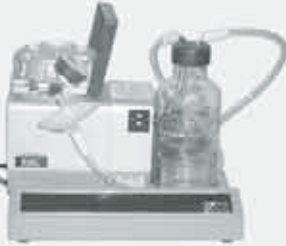
Model M300 Portable Aspirator Lightweight design for general suction, 1/8 hp motor, up to 22 Hg vacuum and includes suction regulating valve
